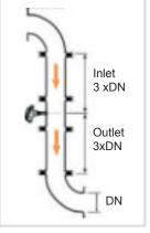
To install a FS 710 a threaded socket is welded onto the pipe and a small hole for the sensor rod drilled. The sensor is fixed on the socket. The rod length should be at least 1/3 of the pipe diameter and the rod must not touch the opposite side. Calibration is done in clean air over a measurement period of 10 min. Sensitivity can be adjusted manually. Retrofits into existing ducts are easy and can be done within minutes.
